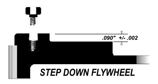
It is important to maintain the proper flywheel step specification. Failure to maintain the proper step specification may result in poor clutch performance, slipage, and/or improper release.
