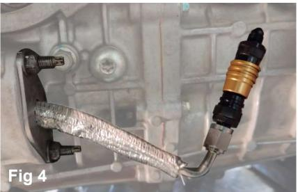
Note: Keep the Hydraulic Quick Disconnect fittings coupled together as shown until the transmission is installed. Doing so will allow the release cylinder to compress and air to escape during the transmission installation.
