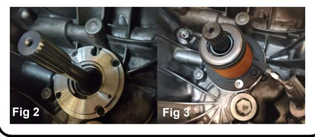
19. Remove the short hydraulic hose from the Release Bearing Cylinder. Install the Centerforce Hydraulic Release Cylinder and Bearing Assembly using the TWO included 6mm bolts. Again, be sure the release bearing hose fitting points to the outside of the bellhousing. Tighten the Bearing Assembly bolts snug using HAND TOOLS only..... torque specifications are 60 inch/lbs. DO NOT over tighten.
