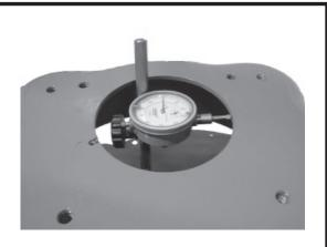
FIRST CHECK BELLHOUSING FOR BORE CONCENTRICITY. INSTALL MAGNETIC BASE TO FLYWHEEL OR PRESSURE PLATE, THEN INSTALL THE INDICATOR TO MEASURE THE BELLHOUSING BORE (SHOWN ABOVE). ROTATE THE CRANKSHAFT AND MARK DOWN THE INDICATOR READINGS (MARKING THE BELLHOUSING WORKS WELL). THE MAXIMUM OUT OF CONCENTRICITY IS .005".
